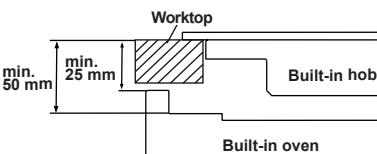
If the oven is installed under a hob, the distance between the worktop and the top panel of the oven must be minimum 50 mm and the distance between the worktop and the top of control panel must be minimum 25 mm.
