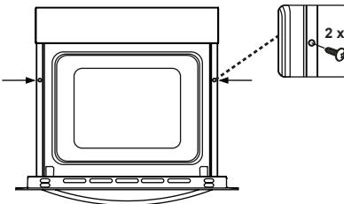
Insert the oven into the cabinet by pushing it forward. Open the oven door and insert 2 screws in the holes located on the oven frame. While the product frame touches the wooden surface of cabinet, tighten the screws.
