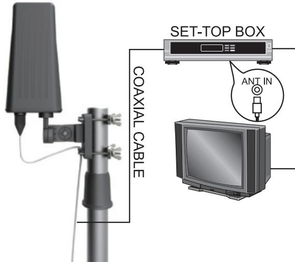
Connect the signal cable from the antenna to the digital receiver, set the receiver to offer power to the antenna and join the TV and the digital receiver.
