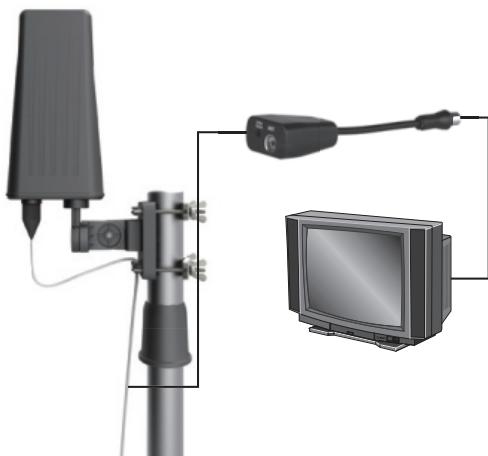
Connect the signal cable from the antenna to the signal input jack of the power supply, connect the power supply output jack to the TV, plug the power adaptor with the power supply and connect to power socket.
