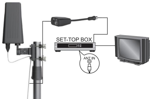
Connect the signal cable from the antenna to the signal input jack of the power supply, connect the power supply output jack to the digital receiver, plug the power adaptor with the power supply and connect to power socket, and finally join the TV and the digital receiver.
