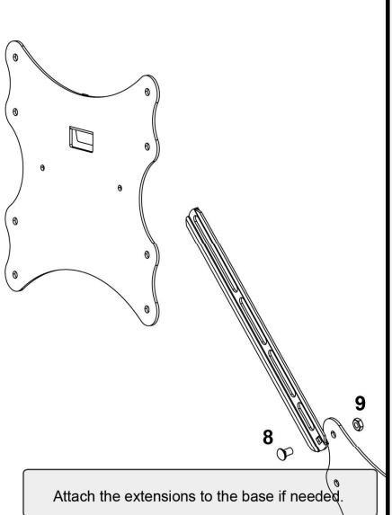
Attach the extensions to the base if needed.
