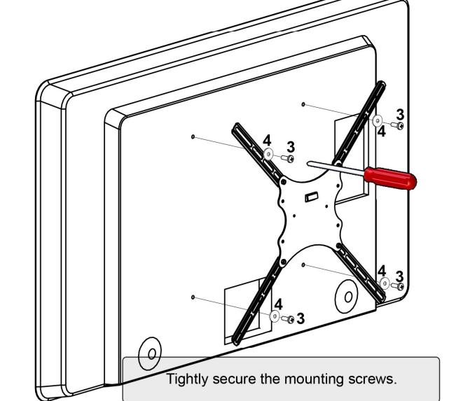
Tightly secure the mounting screws.
