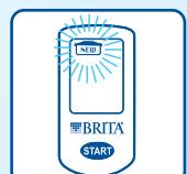
If the empty cartridge symbol "NEW" flashes, you should now exchange the MAXTRA cartridge.
