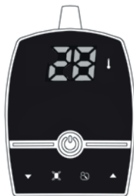
Upper temperature Limit is set at 28°C.
